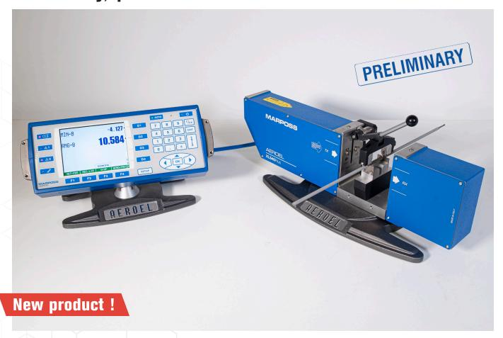
MECLAB.X40 WE is a high-performance tabletop laser micrometer for the off-line measuring of the diameter of the flux coating and it's eccentricity relative to the core wire.
