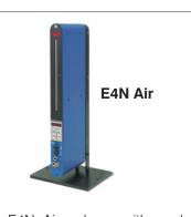
E4N Air column with analog and digital display for manual applications. It can connect one air gauge and elaborate both static and dynamic measurements, featuring also optionally a BCD Relais or an optoinsulated digital output.
