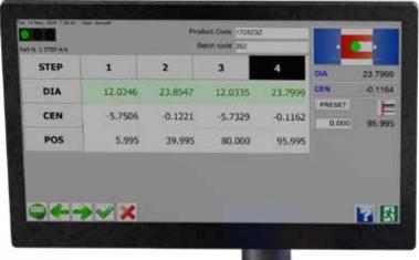
SUPER-MECLAB is an optical micrometer for the shop floor environment, capable to measure diameters with ultra-precision
