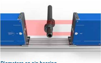
Diameters on pin bearing
