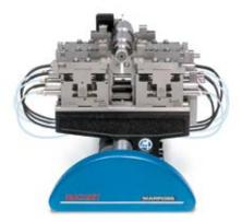
Support bracket L = 200 mm to measure diameters up to 40 mm, with interface for two Quick Block Support bracket L = 250 mm to measure diameters up to 90 mm (without interface for Quick Block)
