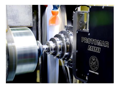
The Protomar Mini gauge is designed to provide fast and reliable measurement across a variety of machining operations.
