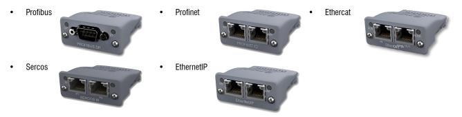
The use of a fieldbus connection means the cabling can be greatly simplified.
