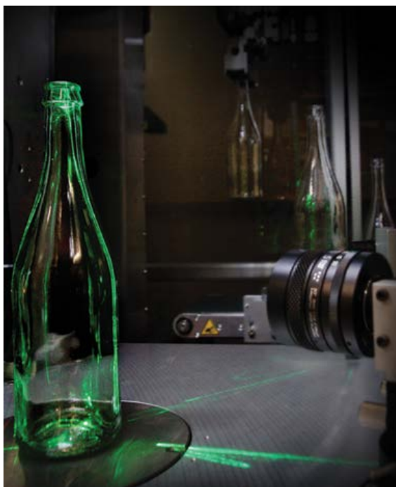
Measuring system for the inspection of the labelling area profile, mounted on the VisiQuick machine.
